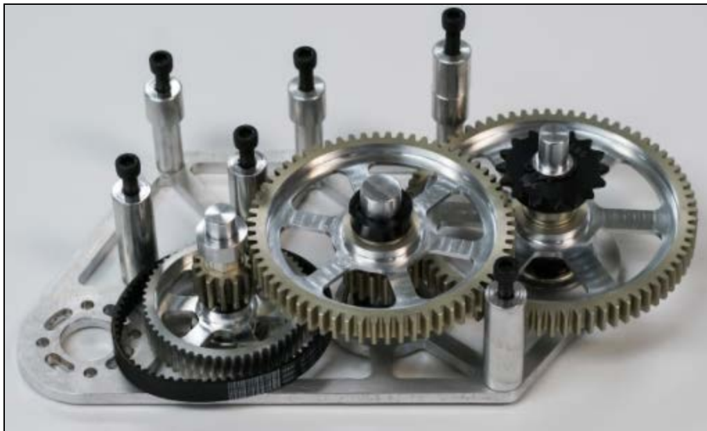
Team 971 Arm Gearbox with Custom Machined Press Fit Hex Shafts.
