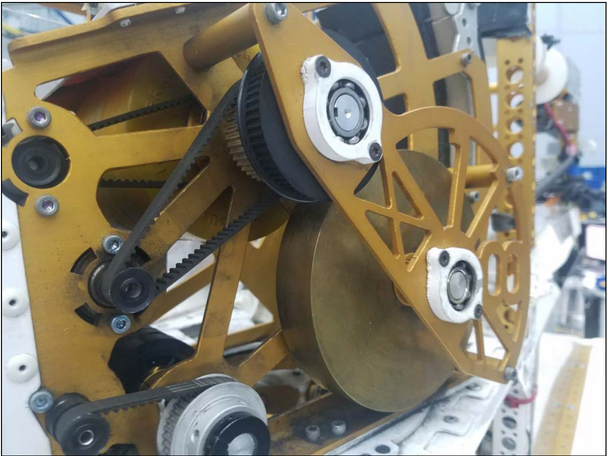
The inertia wheel assembled in the shooter on Team 118's 2017 robot.
