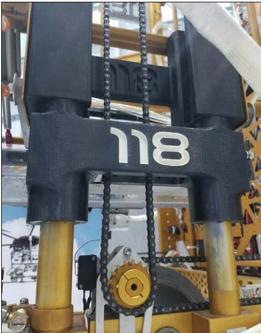
#25 chain run at the bottom of Team 118's elevator from 2015.
