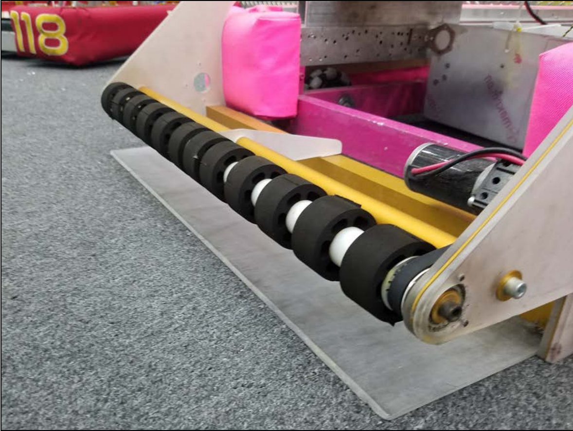
Top roller and dustpan intake on Team 118's driver training robots ; designed to pick up gears from the 2017 game.
