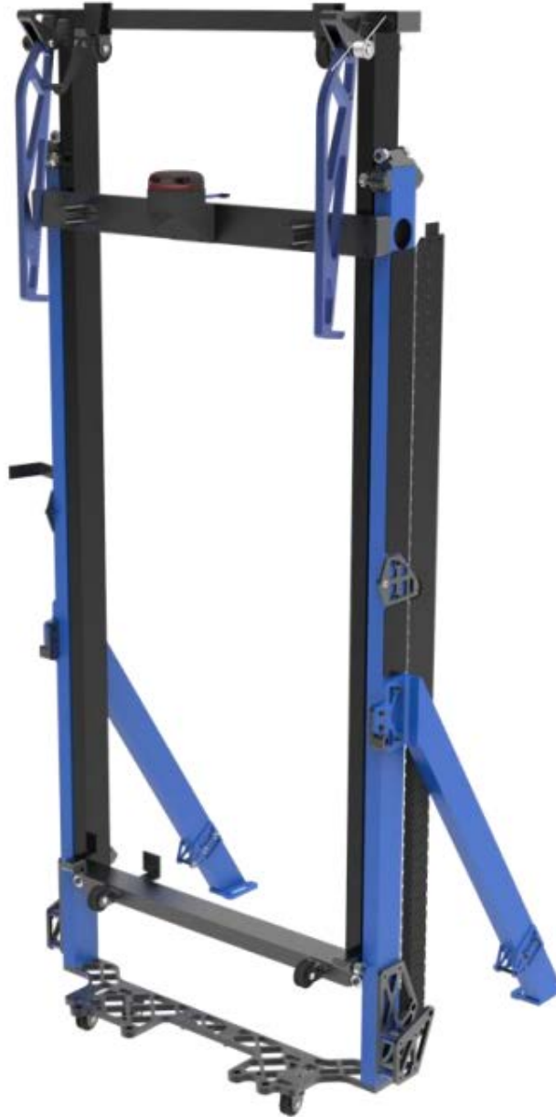
Box tube elevator from Team 254's 2018 robot .
