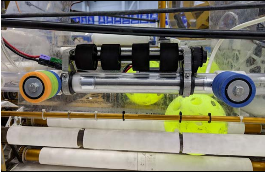
Pneumatic pincher with roller on Team 118's 2017 robot.
