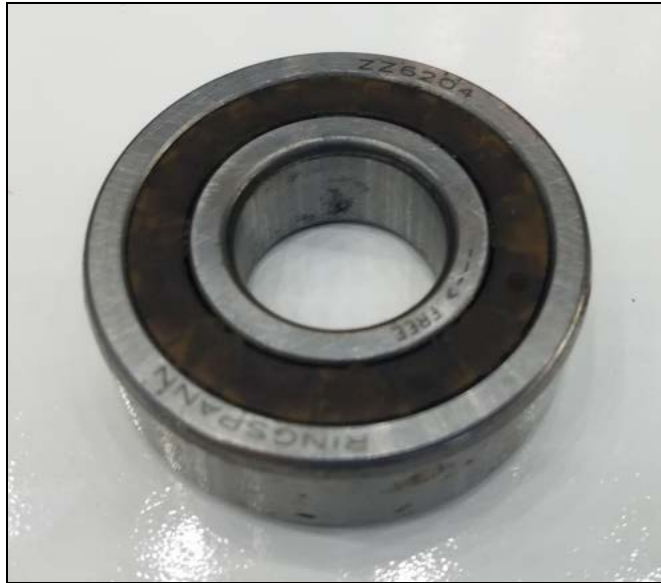
One-way bearing used by Team 118 on their 2017 climber.
