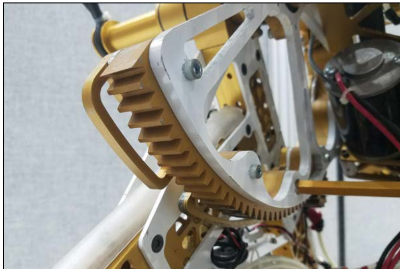
Custom sector gear for the shooter head pivot on Team 118's 2014 robot.
