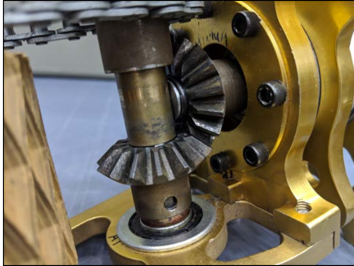
Bevel gears in Team 118's 2008 crab module.
