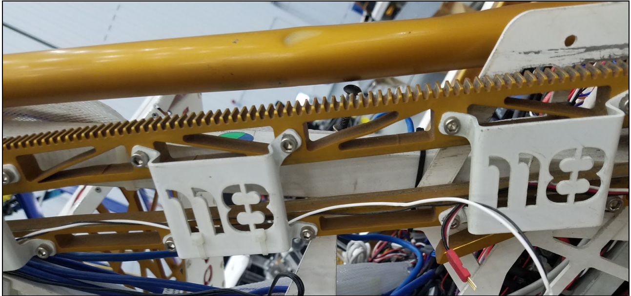
Custom rack gear on the stinger mechanism on Team 118's 2012 robot.
