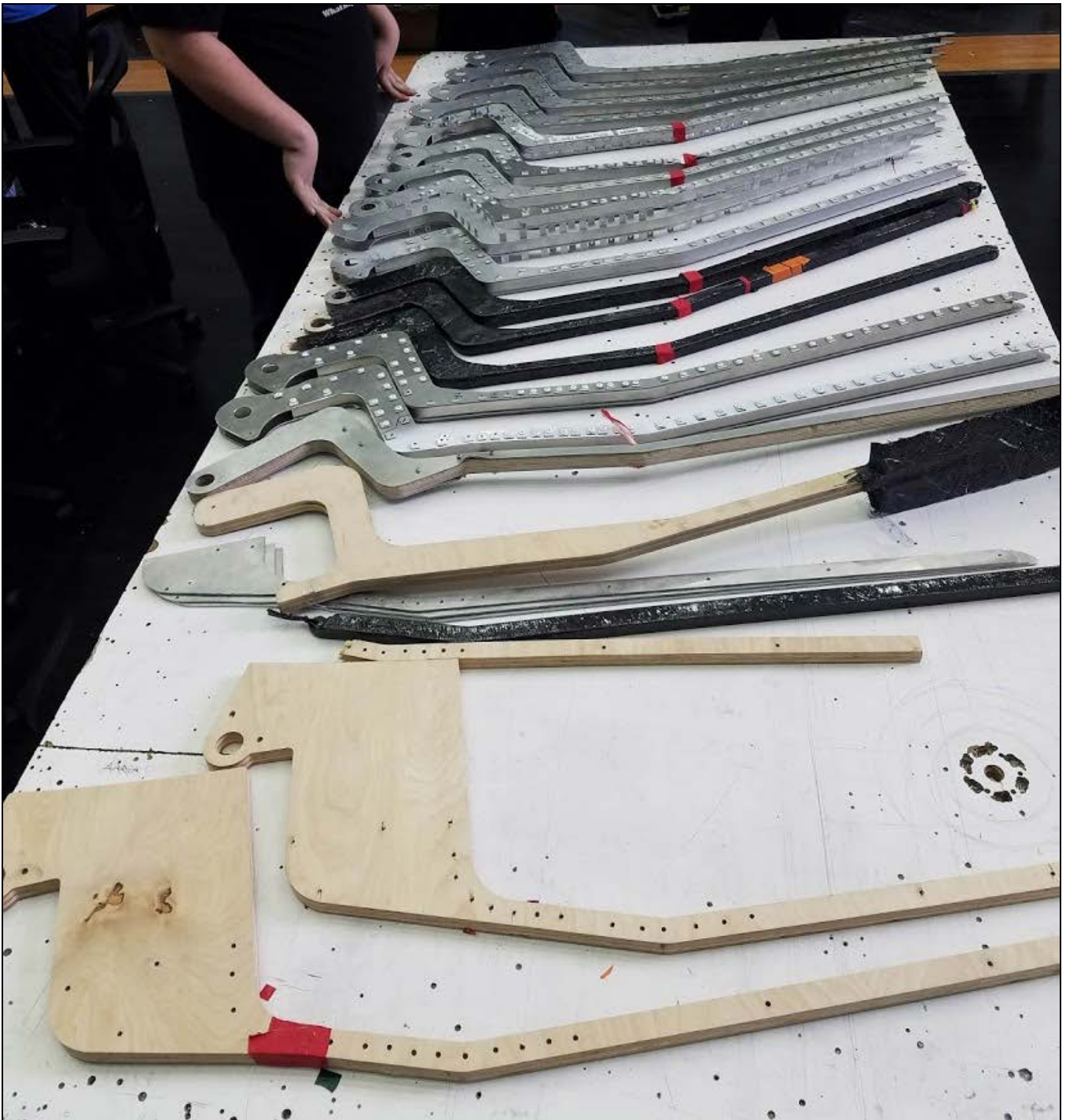
Collection of Prototype and Iterations of Climbing Tines from Team 118's 2018 Robot.
