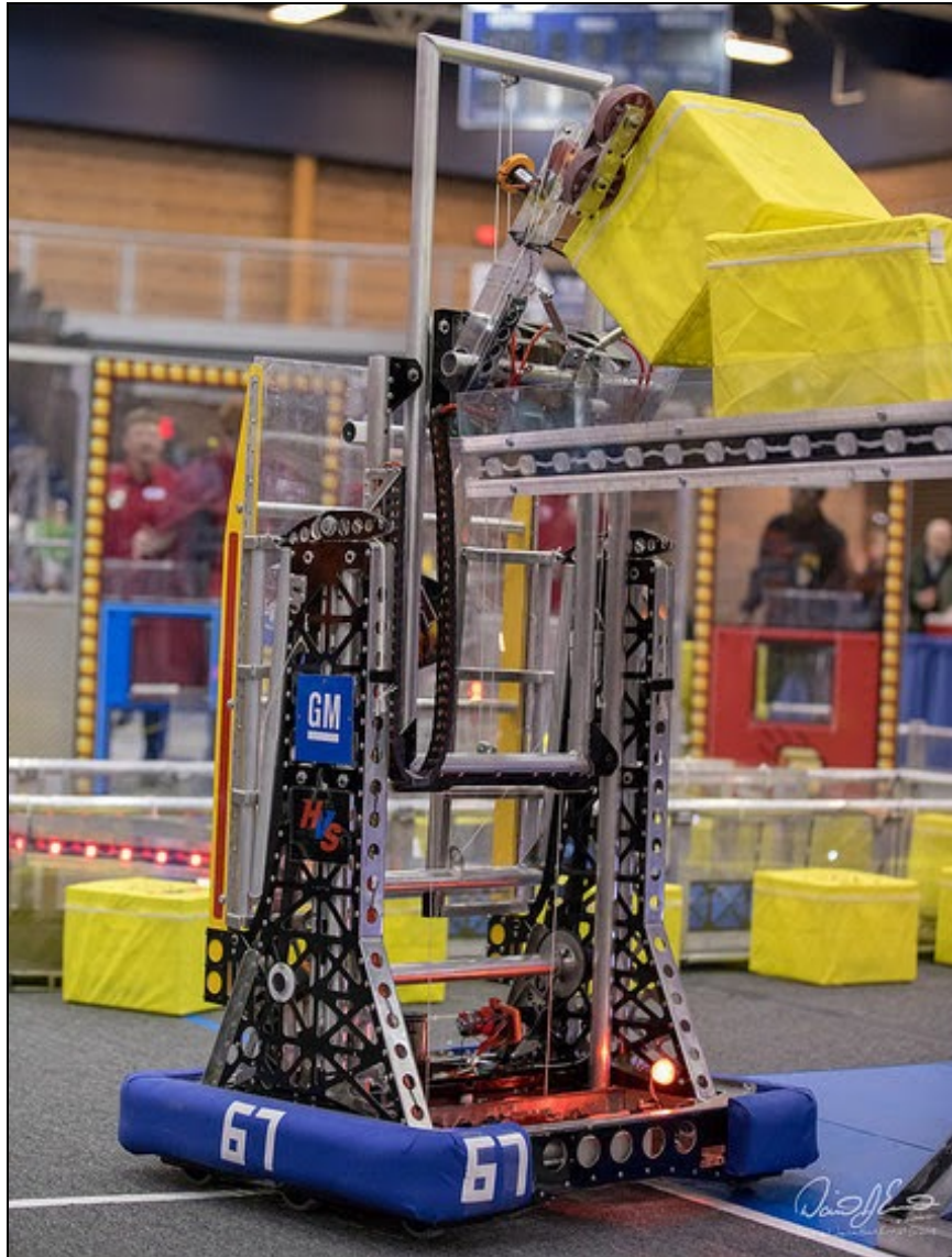
Team 67 is well known for consistently using welded round tube on their robots, as seen at the top of their elevator in this photo.
