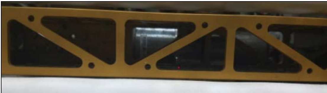
Triangles on the front ladder bar of Team 118's 2017 robot.
