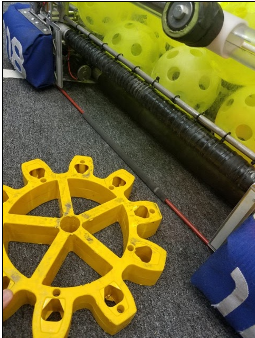
Latex rubber stretched over a fiberglass shaft on Team 118's 2017 gear intake.
