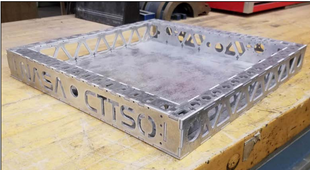
A robot frame built using slots and tabs to create a pseudo-box tube from flat plates.
