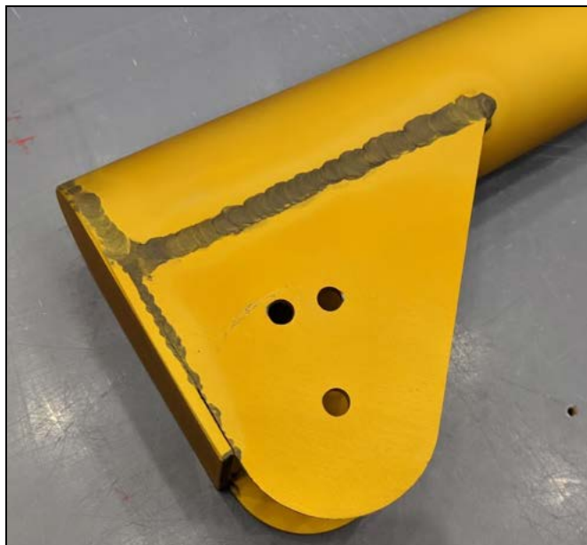
Anodized Assembly with discolored welds with 4043 weld filler.
