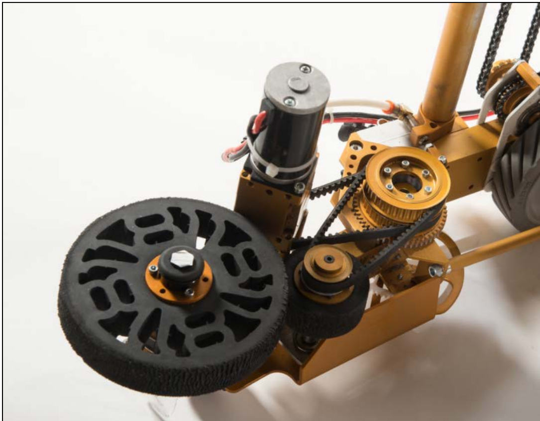
Custom neoprene intake wheels on Team 118's 2015 robot.
