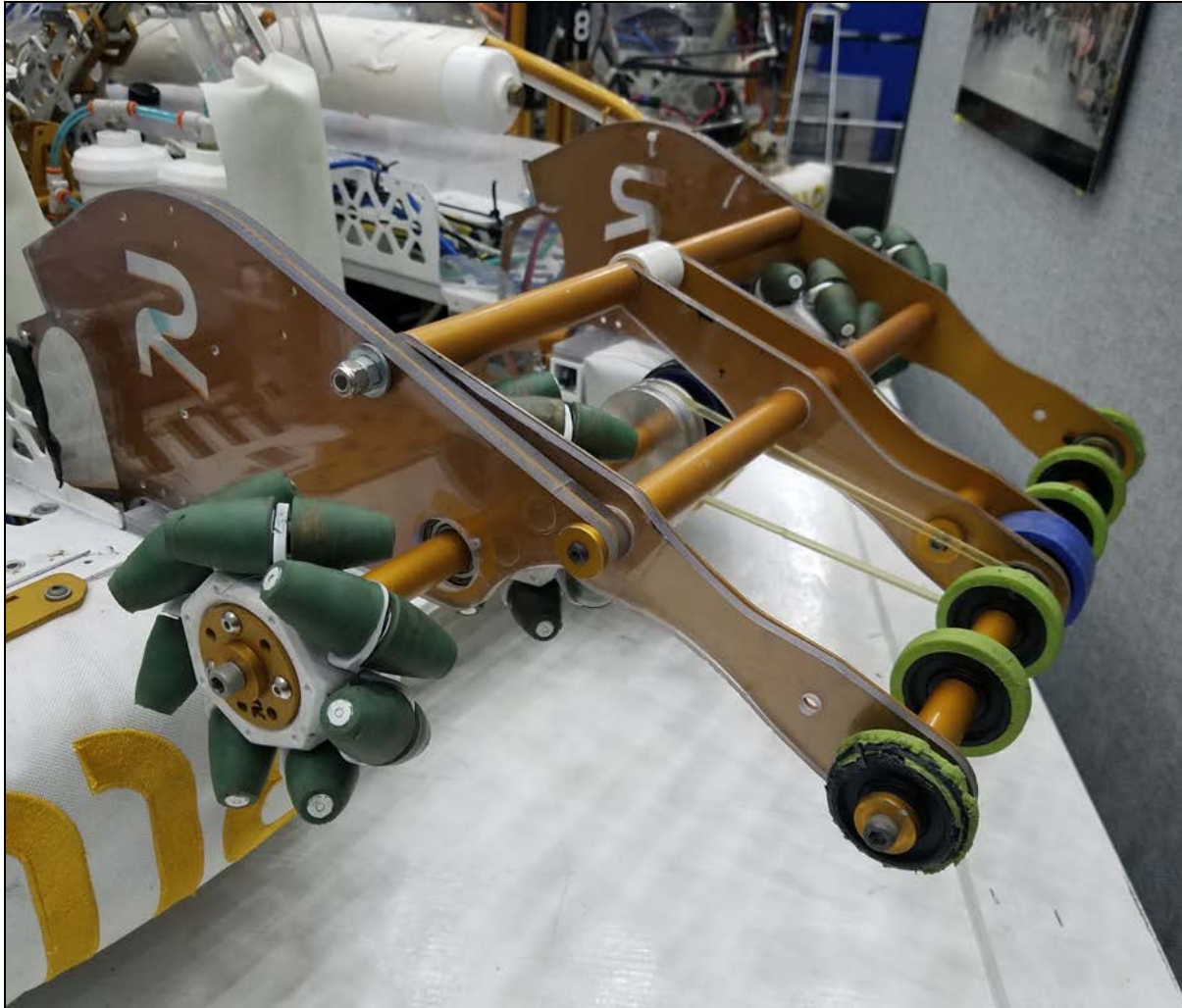
Team 118's top roller intake with mecanum wheels on their 2016 robot.
