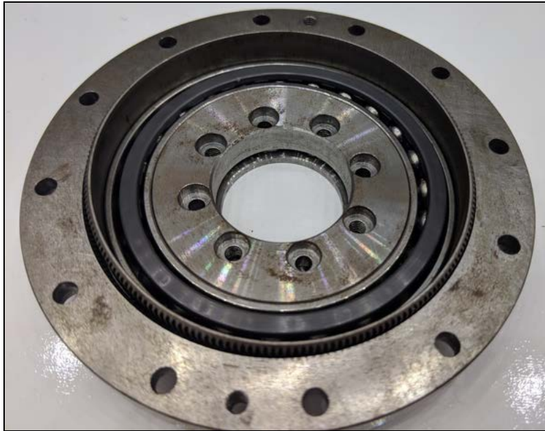
Harmonic Drive used in NASA's Space Exploration Vehicle .
