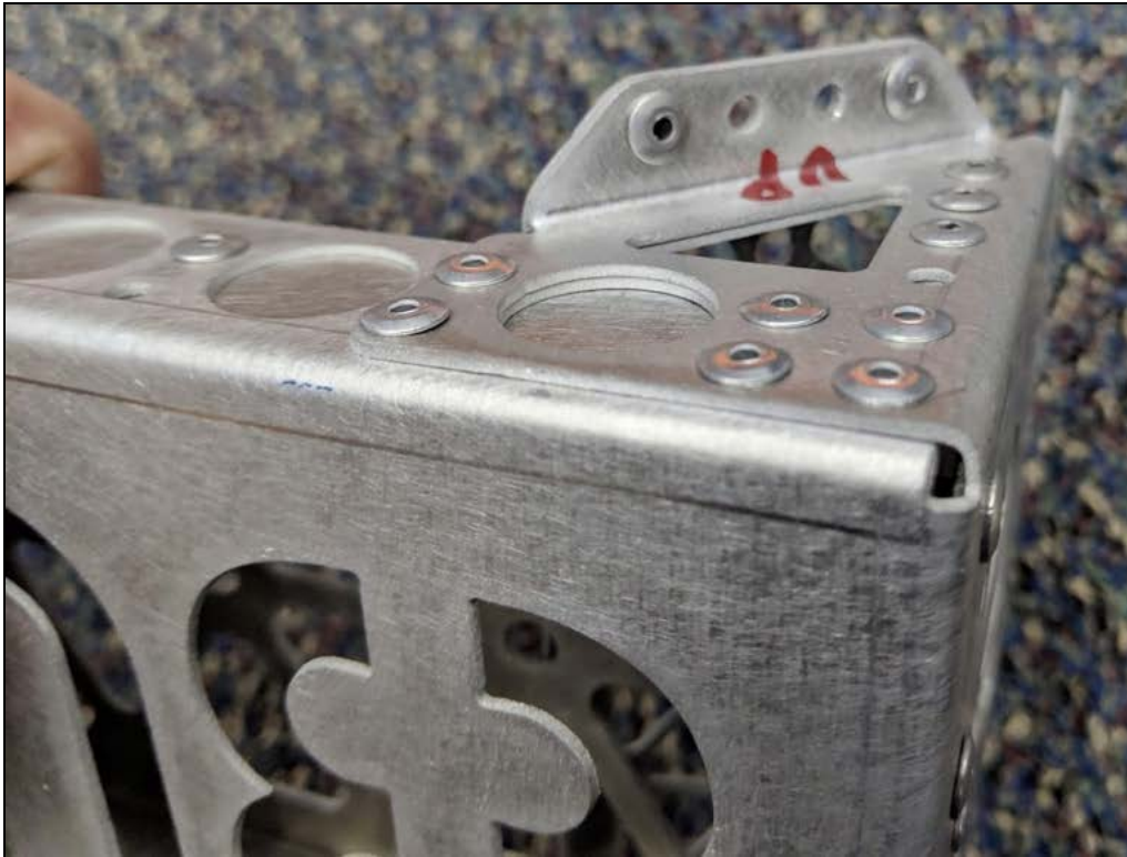
Example of a riveted joint on Team 118's 2019 robot.
