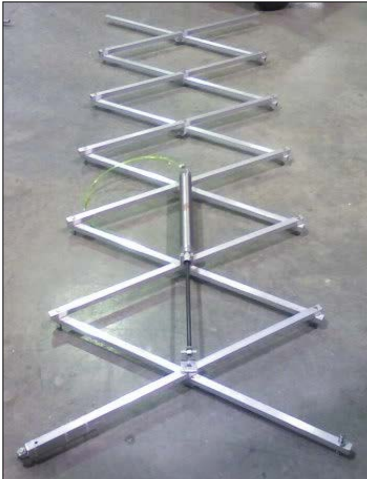
Pneumatically extended scissor lift built by Team 399 .
