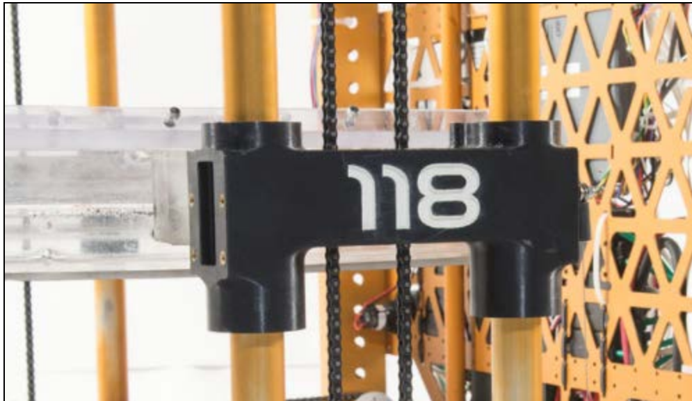
Team 118's 2015 lift trucks printed in ULTEM.
