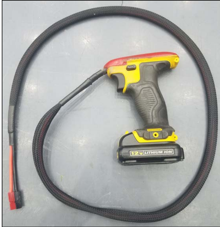
A 12 volt DeWalt drill modified to be a power gun.
